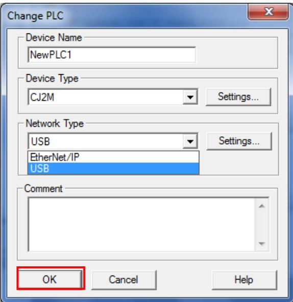
The 'Change PLC' dialog box is shown. It has a title bar with a close button. The 'Device Name' field contains 'NewPLC1'. The 'Device Type' is set to 'CJ2M' with a 'Settings...' button. The 'Network Type' is set to 'USB' with a 'Settings...' button. A pull-down menu is open showing 'USB' selected and 'EtherNet/IP' as an option. There is a 'Comment' text area. At the bottom, the 'OK' button is highlighted with a red box, along with 'Cancel' and 'Help' buttons.
