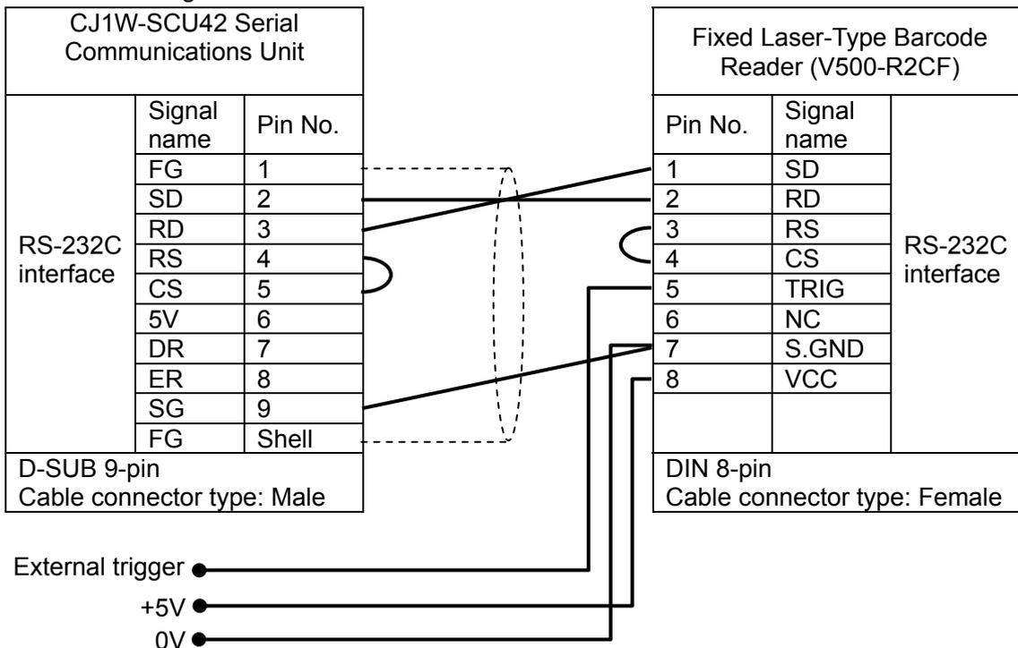
\*The external trigger is not used in this document. Insulate it from other cables.
