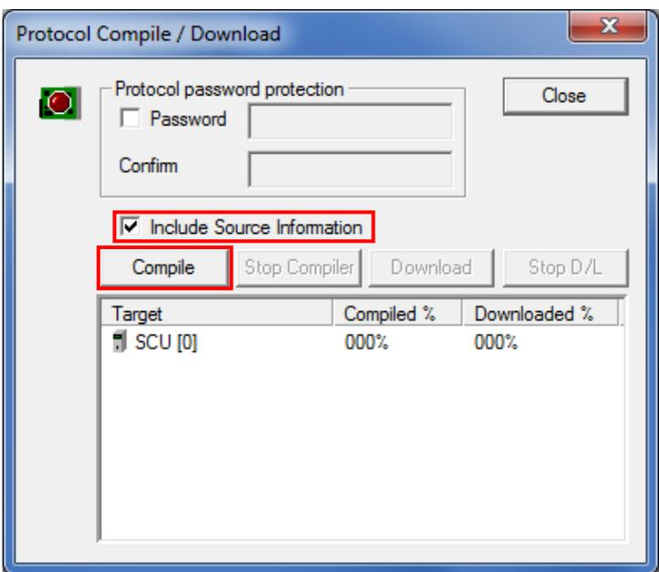
14 When 100% is displayed in the *Compiled %* Column, the compiling operation is completed. After confirming that the compiling operation is completed, click the **Download** Button.
