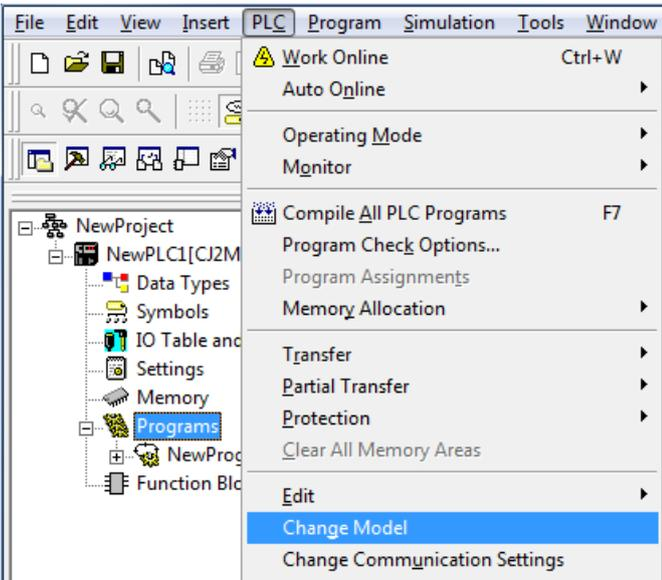
6 The Change PLC Dialog Box is displayed. Select the device type to use from the pull-down list, and click the **Settings** Button.
