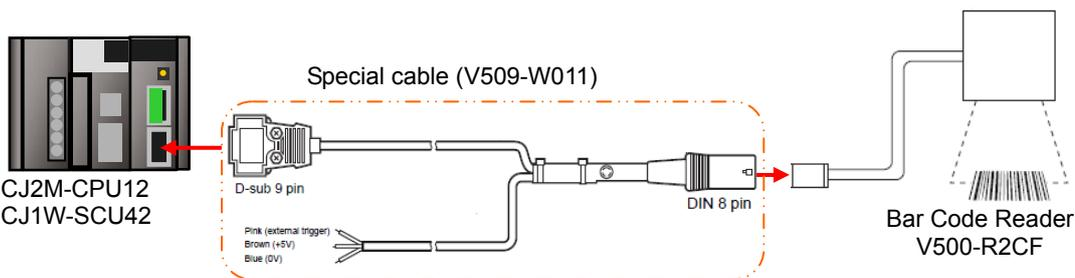
\*The external trigger is not used in this document. Insulate it from other cables.
