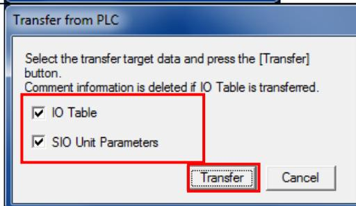
When the transfer is completed, the Transfer Results Dialog Box is displayed. Confirm that the transfer was normally executed by referring to the message in the dialog box.
