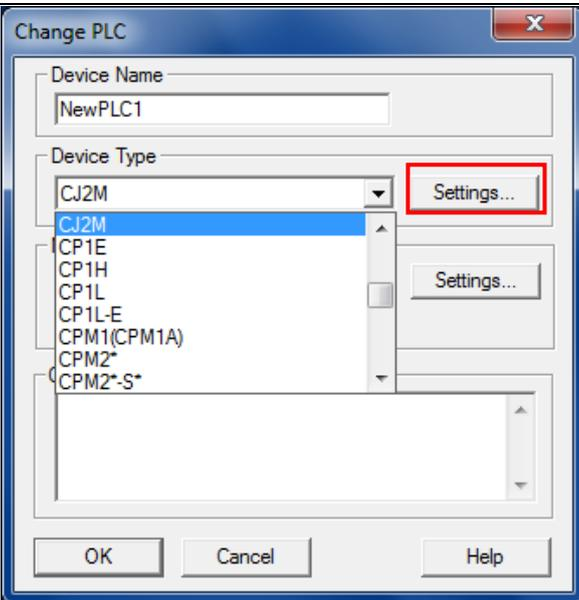
7 The Device Type Settings Dialog Box is displayed. Select the CPU type to use from the pull-down list, and click the **OK** Button.
