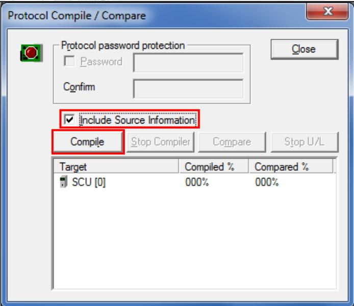
19 When 100% is displayed in the *Complied %* Column, the compiling operation is completed. After confirming that the compiling operation is completed, click the **Compare** Button.
