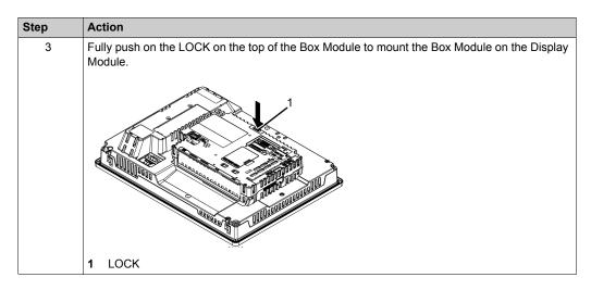
**NOTE:** For instructions on how to mount the Display Module to the panel, refer to Installing to the Panel (see page 112).
