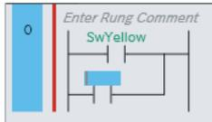
An N.O. input is inserted in an OR structure.
