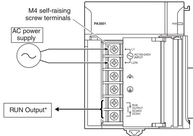
\* The RUN output is ON when the CPU Unit is in RUN mode. It is OFF when the CPU Unit is in PROGRAM mode or when a major fault level Controller error occurs.
