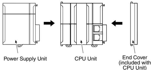
After joining the connectors between the Units, use the sliders at the top and bottom of each Unit to lock the Units together. Lock the sliders firmly into place.
