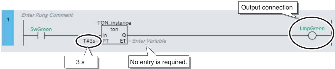
Enter the input parameter for input variable *PT*. We want the indicator to light after three seconds, so enter *T#3s* here.
