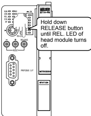
8) Press the RELEASE button again and hold it until the REL. LED turns off. \*5
