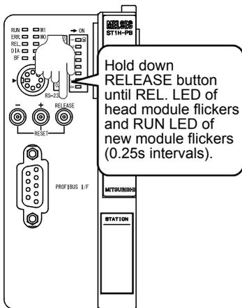
7) After mounting the new slice module, press the RELEASE button of the head module until its REL. LED flickers. When the REL. LED flickers, the head module starts writing the saved user parameters and command parameters into the new slice module. When the following conditions are confirmed, release the RELEASE button.
