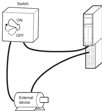
6) After mounting a new slice module, connect it to the external device. For details, refer to "External device connection and disconnection procedures for online module change".
