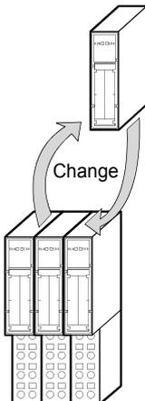
4) Remove the slice module to be replaced from the base module.
