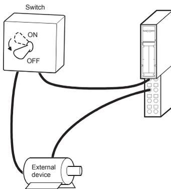
3) Disconnect the external device from the slice module to be replaced online.
