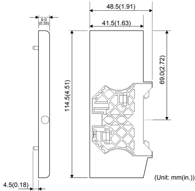
\*1. In the above drawing, the end bracket is mounted on the end plate.
