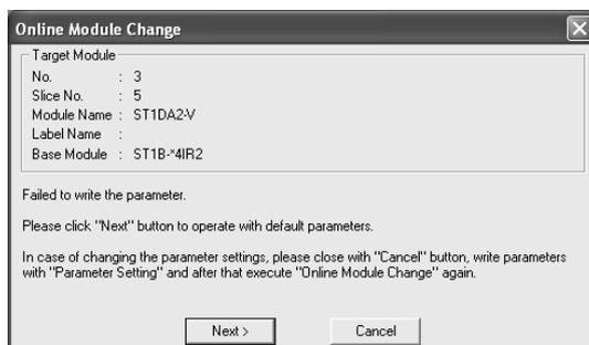
When the user parameters and command parameters could not be read from the old slice module by the operation in step 3), the REL. LED and ERR. LED of the head module turn on and the screen shown on the left appears on GX Configurator-ST.
