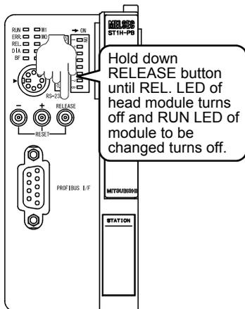
2) Keep pressing the RELEASE button of the head module until its REL. LED lights up.
